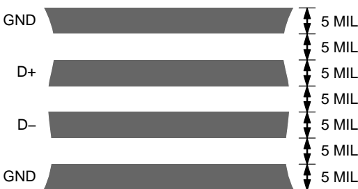
Figure 21. Typical Arrangement of Signal Tracks
